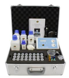
Through a combination of iron test and BN measurements with Vecom Marine's TEST KIT TWIN CHECK 4.0 proper lubrication of cylinder components and therefore optimal engine performance can be ensured.
