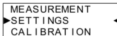
3. In the “SETTINGS” menu, please complete all necessary settings such as date, time and the name of the parameter to measure (water-in-oil or base number). This will help to always ensure the accuracy of information with proper record keeping and trending of oil analysis data.
