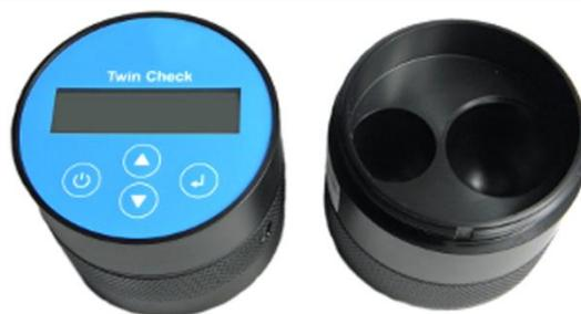
2. Fill the larger chamber of the reaction vessel with the thoroughly shaken ALCA solution up to the lower marked point. In case of accidental solution spill into the smaller chamber of the reaction vessel, please, wipe it away immediately with a soft cleaning cloth.
