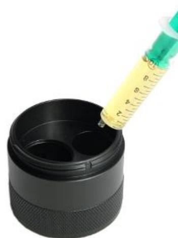
4. Close the lid of the reaction vessel carefully. Make sure that the liquids do not mix yet.
