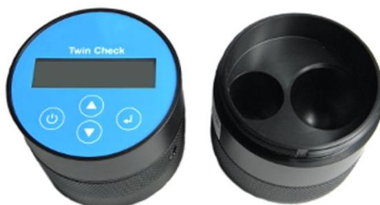
2. Fill the larger chamber of the reaction vessel with the prepared solution up to the lower marked point. In case of accidental solution spill into the smaller chamber of the reaction vessel, please, wipe it away immediately with a soft cleaning cloth.
