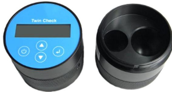
2. Fill the larger chamber of the reaction vessel with the thoroughly shaken ALCA solution up to the lower marked point. In case of accidental solution spill into the smaller chamber of the reaction vessel, please, wipe it away immediately with a soft cleaning cloth.
