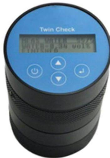
**Note:** The measuring time can vary significantly starting from two minutes (no water detected in the oil sample and the measurement gets cut off automatically) to maximum twenty minutes (maximum total reaction time). The measuring range covered is **0 – 1.0 vol. % H<sub>2</sub>O**.
