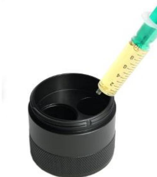
4. Close the lid of the reaction vessel carefully. Make sure that the liquids do not mix yet.
