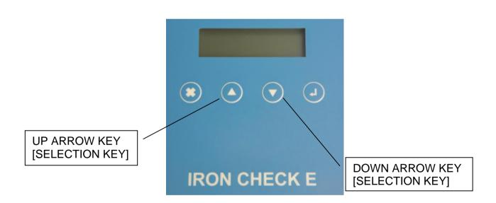
Once the oil sample is added, chemical reaction occurs and automatic electronic evaluation process of the iron content starts. As the measuring process is fully automatic, no manual intervention is required.
