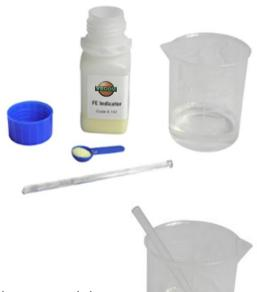
3. With the help of the glass rod, the distilled water and the FE Indicator powder should be thoroughly mixed until clear light-yellow solution is obtained.
