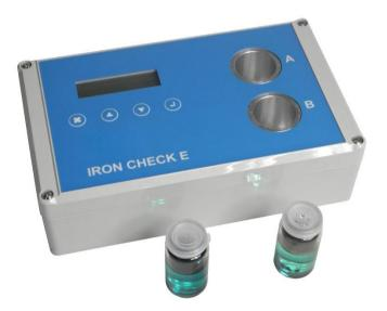
**As an example only**, please see the liquids with different shades of blue color which directly depend on the amount of iron concentration in cylinder drain oil samples.
