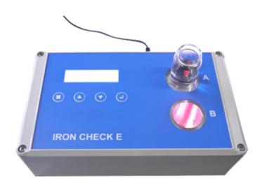
**Note:** Both chambers A and B of the IRON CHECK E can be used simultaneously in case two or more oil samples have to be tested to determine total iron content. This advantage enables to save time.
