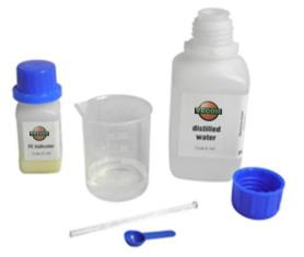
2. One full measuring spoon of the FE Indicator powder has to be added to the distilled water in the plastic beaker.
