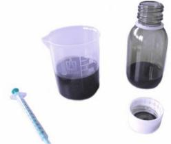
Draw 0.5 ml of the cylinder drain oil with the help of a syringe.
