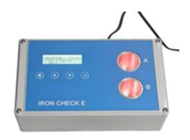
The display of the test unit IRON CHECK E shows gradual temperature increase up to the default temperature of 70°C.
