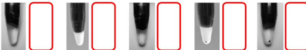
Visual quantification by means of Comparison Chart TEST KIT CAT FINES CHECK
