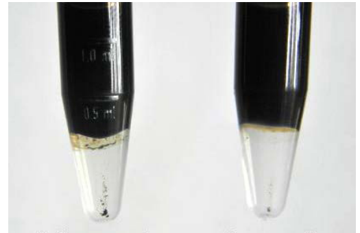
Left: before separator Right: after separator
