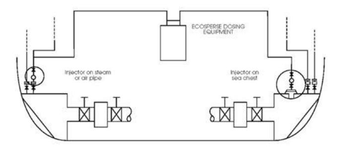
Typical installation of ECOSPERSE dosing equipment. Injection point can be fitted also in the sea chest strainer box.
